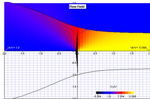
Figure 16: Flow field of the propeller
