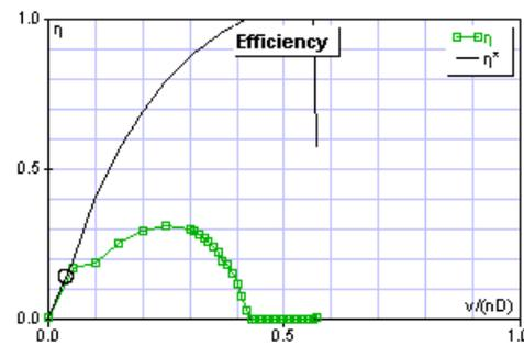
Figure 13: Graph of efficiency VS advance ratio
